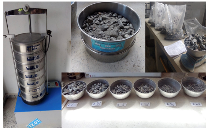
Figure 6. Granulometry test: Mechanical sieve, sieves and samples classified by size
