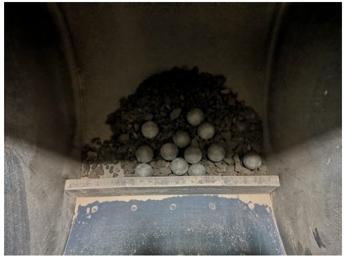
Figure 7. Wear test on the Los Angeles machine This figure shows the spheres that simulate the abrasive load on the material, the material before the test and the disintegrated material once the test is performed.
