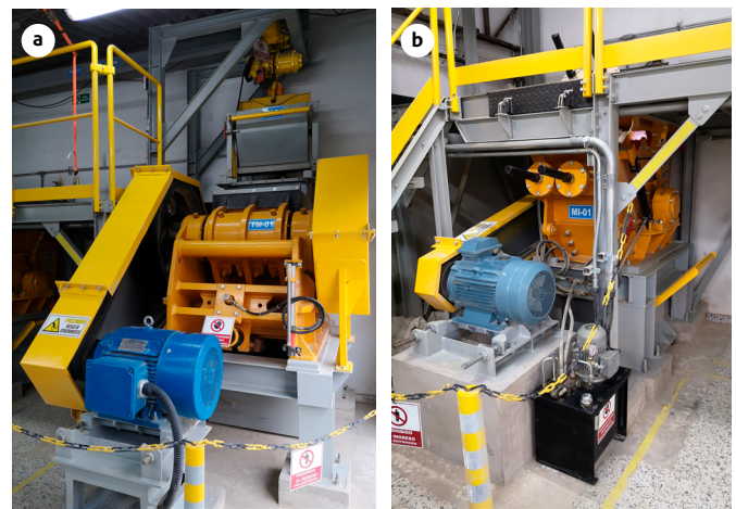
Figure 4. Primary and secondary crushing laboratory of the Servicio Geológico Colombiano a) Jaw crusher; b) impact mill.
