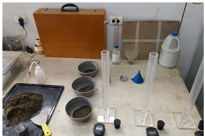
Figure 8. Sand equivalent test Specimens in the same test to determine an average value of sand equivalent readings
