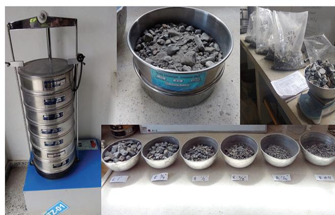
Figure 6. Granulometry test: Mechanical sieve, sieves and samples classified by size
