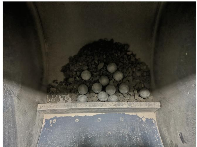
**Figure 7.** Wear test on the Los Angeles machine
