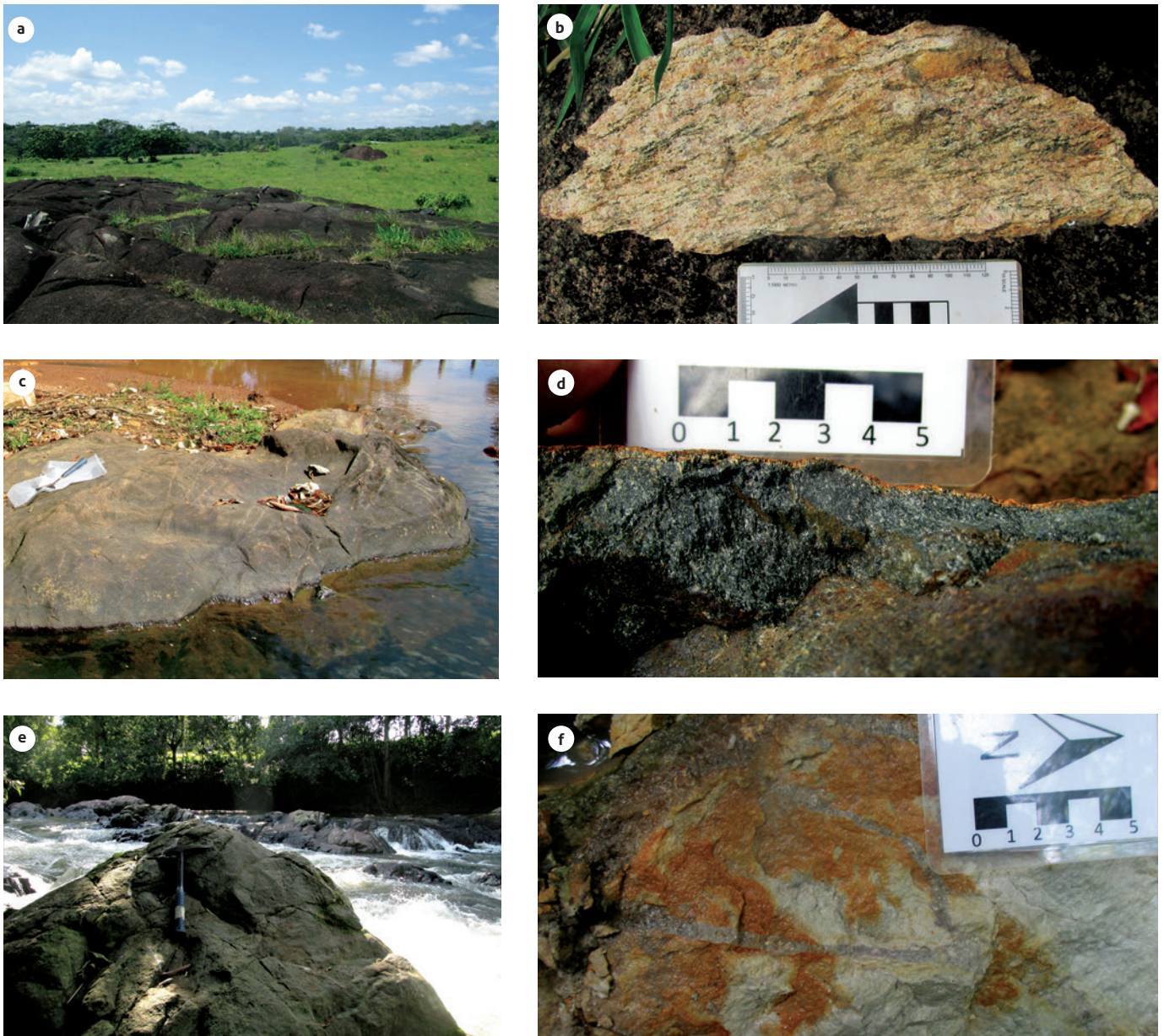
Figure 3. Texture and lithology of the rocks of the Guaviare Complex in macrosamples a and b) Quartz-feldspar gneiss. c and d) Medium-grain amphibolite. e and f) Quartzite; note the quartz veins
