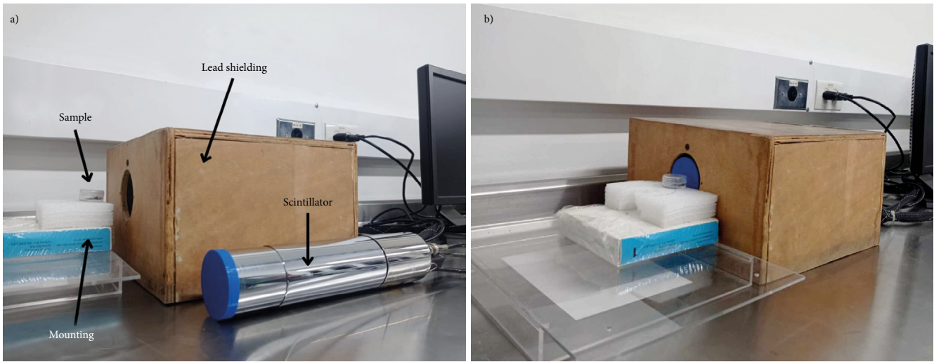
Figure 1. a) Scintillator, lead shielding and sample mounting. b) Experimental setup for measurement
